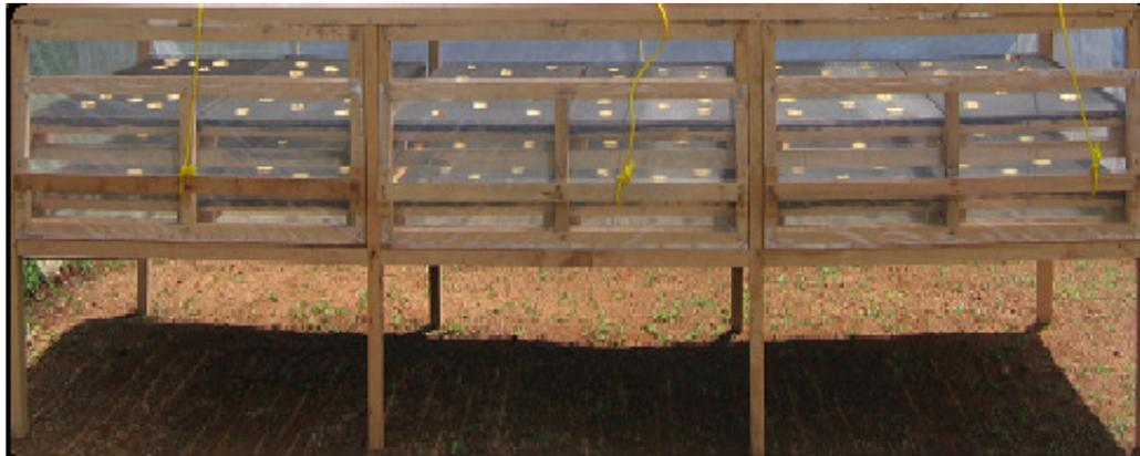
**Figure 1.** NRI-modified Kawanda solar cabinet dryer (front view) constructed at JUCAVM, Ethiopia. The dryer consisted of a main frame with eight supporting legs, incorporating the drying chamber covered with transparent polyethylene sheet. The drying chamber was 4.4 m long x 1.5 m deep x 0.8 m high overall and contains 12 trays to provide a total drying area of 10 m<sup>2</sup>.
